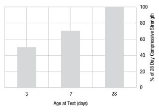
Cement Content = 320kg/m<sup>3</sup> Slump = 80mn
