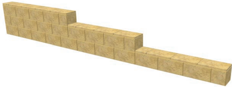
Stepping down using a half corner
